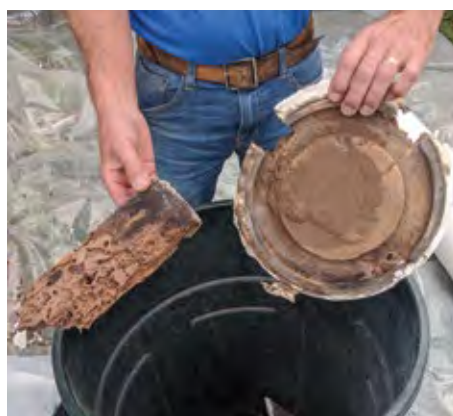
Elements of the columns showing extensive insect infestation.
